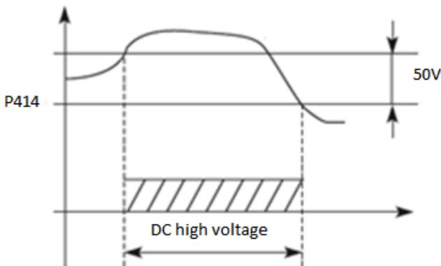
If the P414 value is too high, the DC voltage may be too high and may cause switch ON of the inverter protection. If the P414 value is too low, the braking resistor may be too hot.
