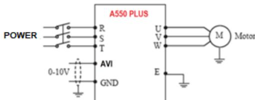
Explanation: the output frequency is controlled via the AVI terminal (0-10V).
