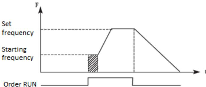
The starting frequency is the initial frequency at the start of the inverter. For equipment with a heavy load or requiring a large starting torque, the starting frequency is increased. However, if the starting frequency is too high, it may cause the overload protection to activate.
