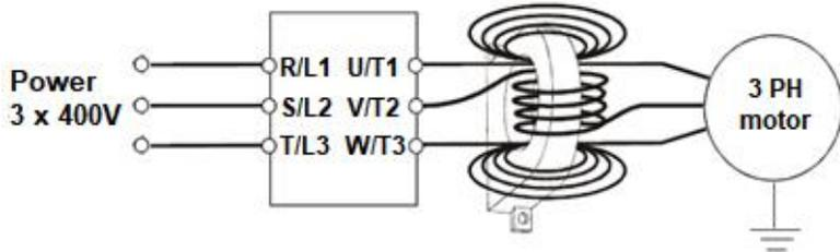
(8.2) Techniques to reduce noise that enters the converter and causes it to malfunction.
