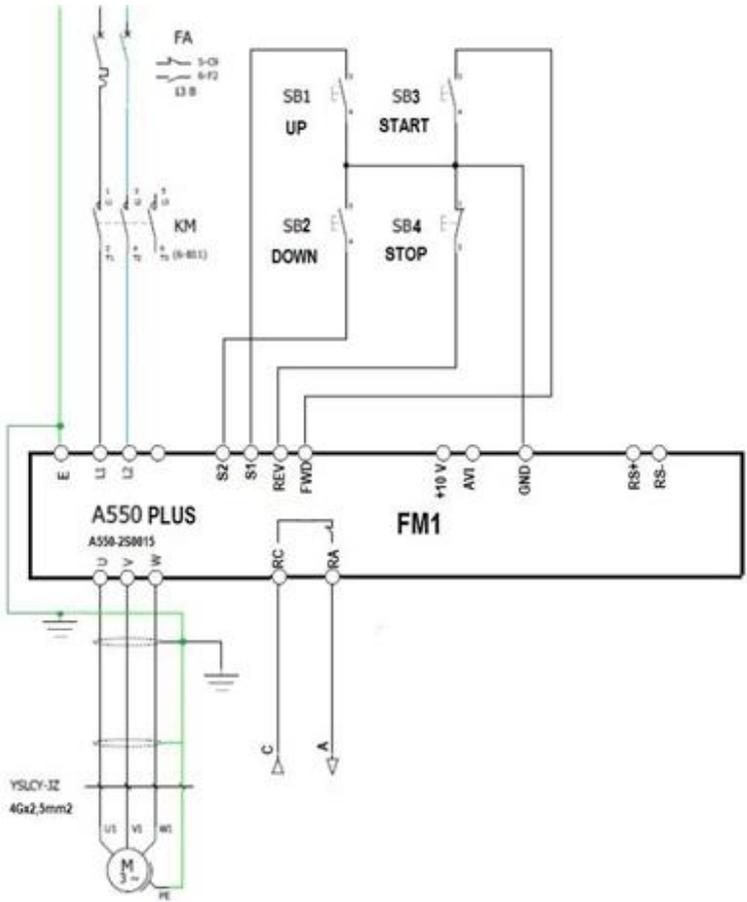
**9.11 Example No.11: Connection of external control with connection of PTC protection of the electric motor and with connection of EMS (CENTRAL STOP) safety button**
