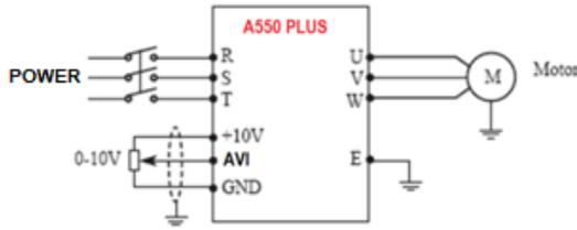
Explanation: the control output frequency of the inverter is controlled using the AVI voltage signal from an external POT (eg 10 kΩ). Position J2 = V
