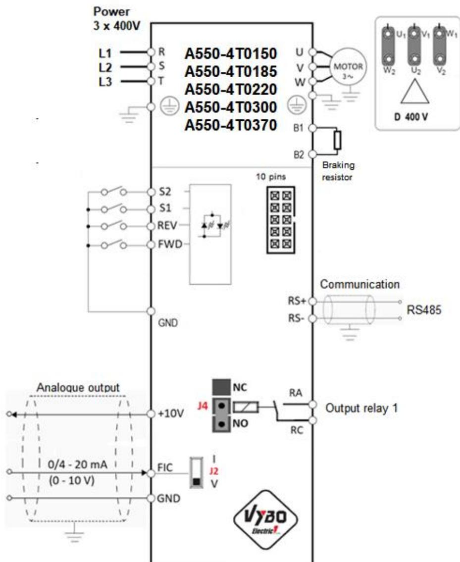
4.6.1 Frequency inverter control terminals A550 Plus model C
