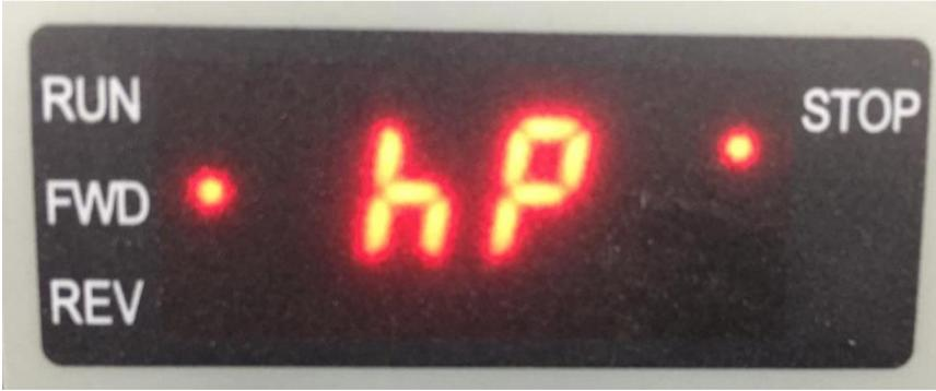
During PID operation (constant pressure control), you can use the up arrow (button) to add the desired set pressure, and conversely, use the down arrow (button) to decrease the value of the desired pressure even during operation.
