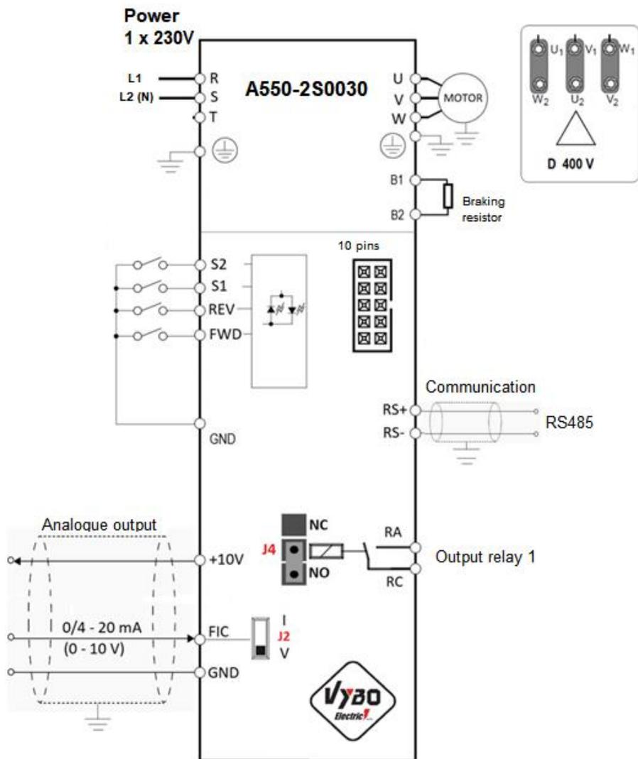
4.5.1 Frequency inverter control terminals A550 Plus models B4T and B2S
