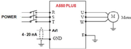
The output frequency of the inverter is controlled by an external current signal (4-20 mA), which is fed to the inverter through the AVI terminal (position J2 = I).
