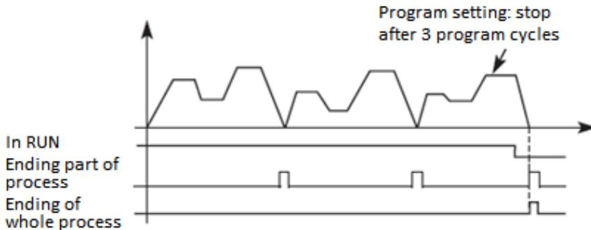
13: Indication of the end of the process. In PLC operation mode, the inverter will generate this pulse signal when the inverter has finished the whole program.
