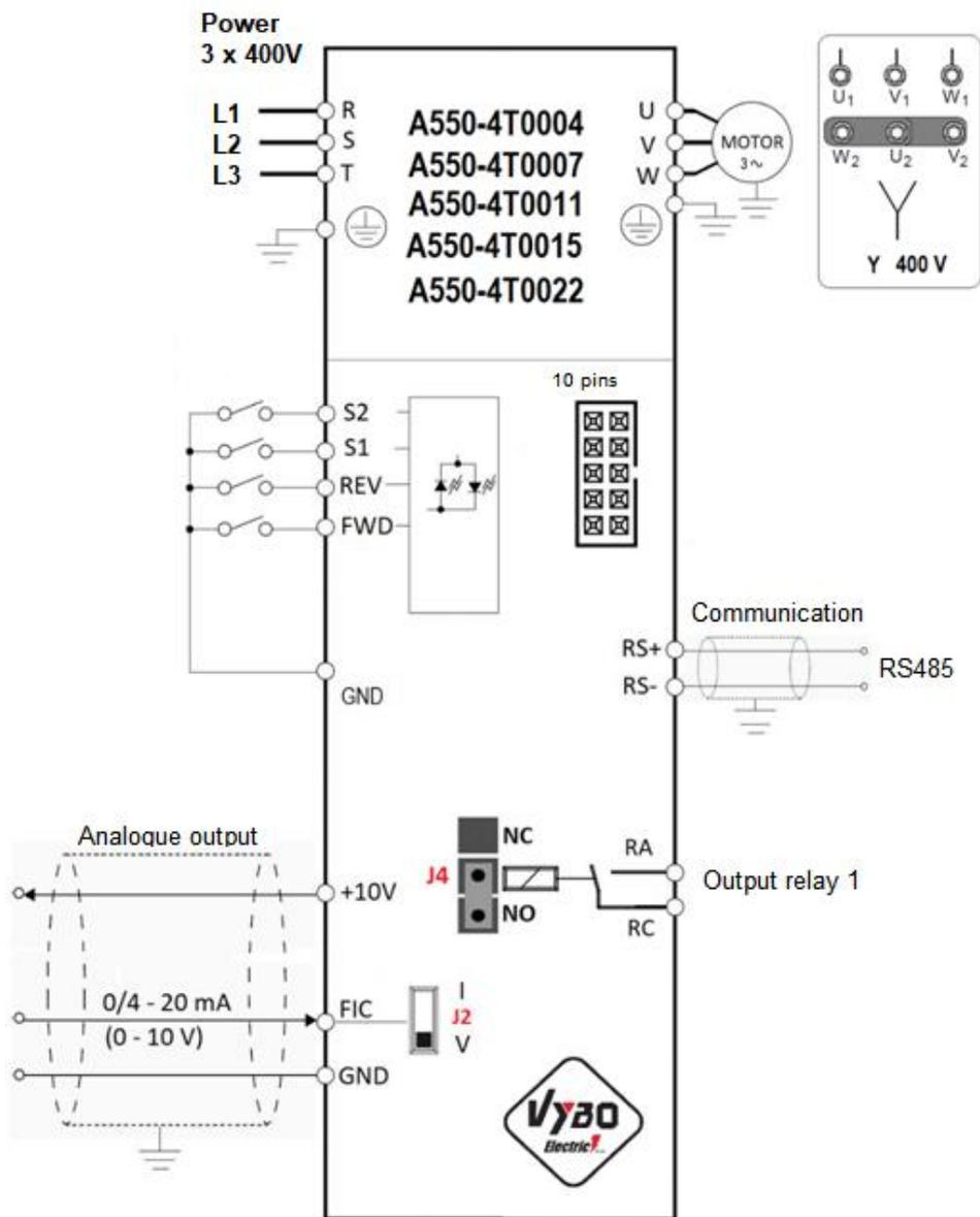
**4.3.1 Frequency inverter control terminals A550 Plus models A2S; A2S...S and A4T**
