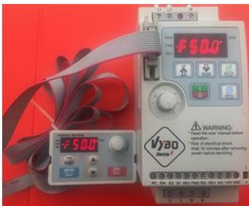
Connected external control panel
