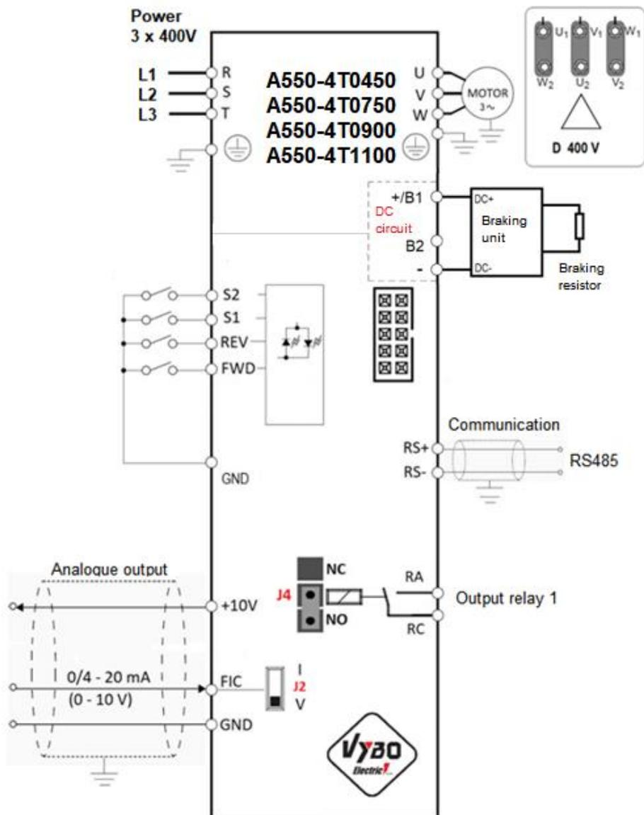
4.7.1 Frequency inverter control terminals A550 Plus model D
