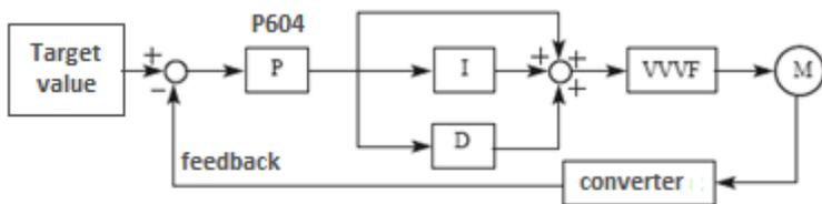
Set the upper limit value. If the feedback value exceeds the set value, an alarm will be triggered. The maximum input (20 mA / 10 V) of the measured value (terminal AVI) corresponds to 100%.
