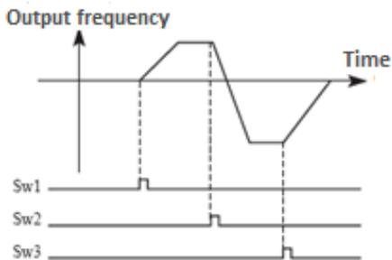
**3: Three-wire mode 2** - In this mode, Sn enables command execution. The CHOD command is given by the Sx signal and the direction is determined by the Sy signal.
