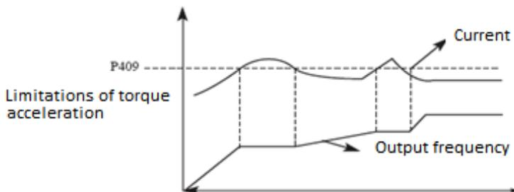
100% of the current is the rated current of the inverter; if P409 is set to 0 then the torque limitation is inactive and does not have a protective function.
