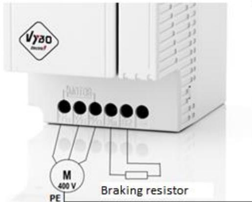
P9.03=0 (activates the brake resistor)
