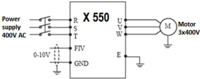
Explanation: the output frequency is controlled via the AI / FIV terminal (0-10V).
