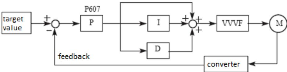
General control method for PID control:
