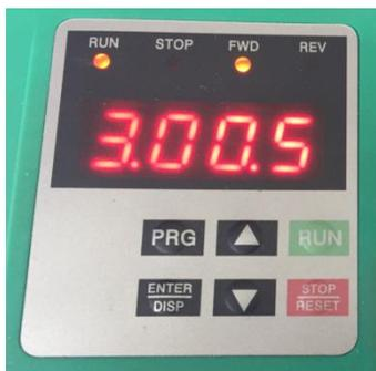
The "SLP" display has changed to "3.0 0.5" the inverter display shows the value of the required pressure 3.0 bar on the left and the pressure value in the system on the right, i.e. 0.5 bar. The inverter has been activated and the pump motor starts to reach the required pressure of 3.0 bar.
