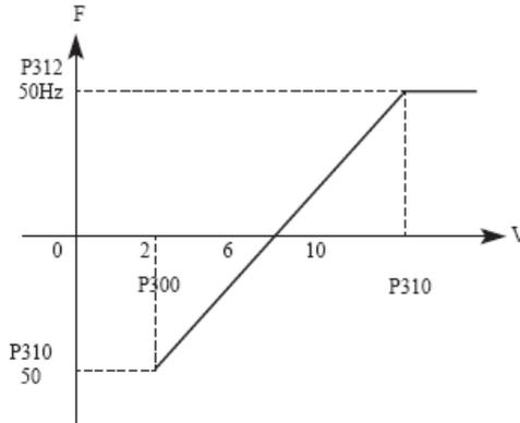
P300 = 2, minimum voltage input FIV: 2V (the inverter considers signals below 2V as invalid signals);
