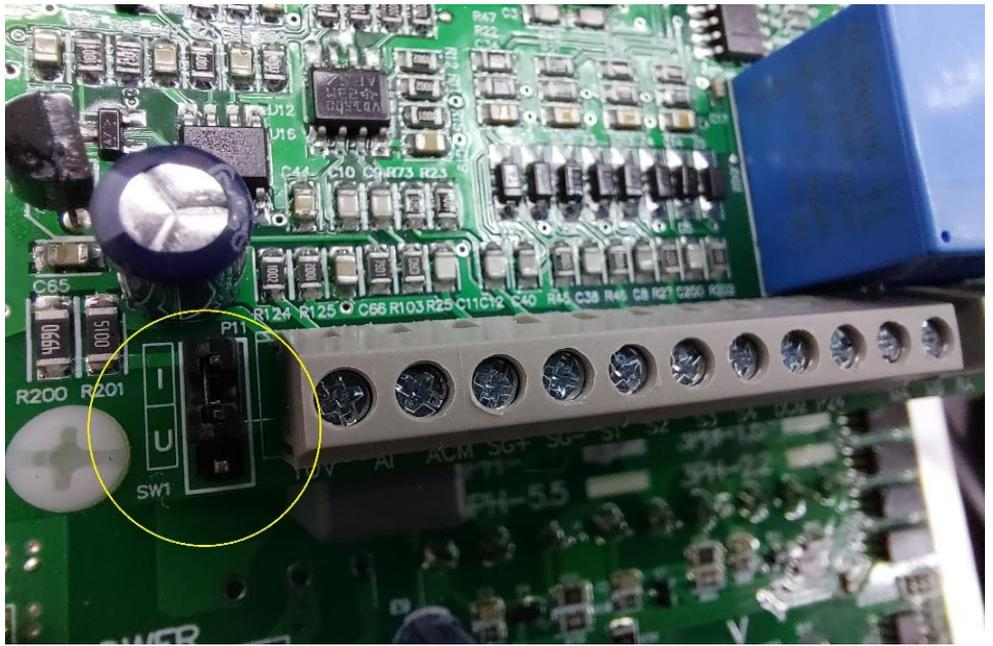
Attachment No 6 Location of switch SW1 on X550 models above 7.5 kW
