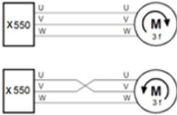
The direction of rotation of the motor can be changed by swapping the two output lines on the frequency converter or the motor.
