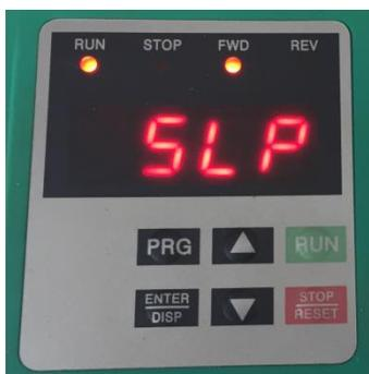
The display shows SLP (sleep), this means that the inverter has reached the required set pressure and if the pressure in the system does not decrease (e.g. there is no water intake), the inverter goes into "sleep" mode.
