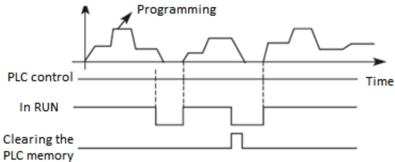
During the running of the PLC program, due to a fault or stop, the frequency inverter will automatically record the program status, after removing the fault and turning on the inverter again, the frequency inverter will continue to operate according to the program. If memory clearing is enabled, the program will be reset and the drive will start from the beginning.
