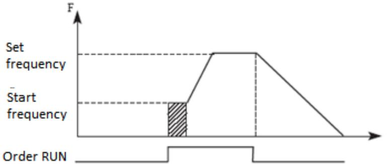
The starting frequency is the initial frequency at the start of the inverter. For equipment with heavy load or fast fast torque, it increases the starting frequency. However, if the trigger frequency is too high, it may cause the over-protection to activate.
