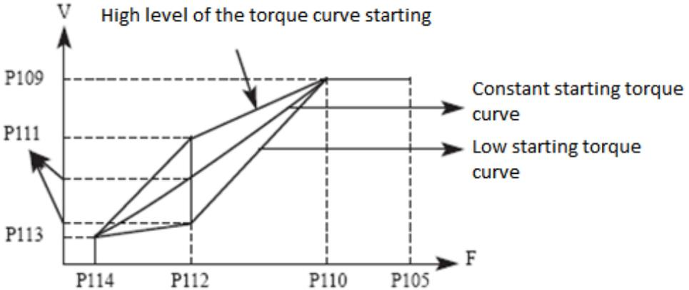
High level of the starting of the torque curve: application for heavy loads and loads that require a high starting torque.
