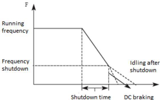
As for the stop mode after reaching the stop frequency, you can choose DC brake and other options. If you do not select DC braking, the motor will automatically stop in coasting mode.
