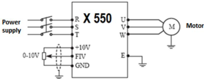
Explanation: the control output frequency of the inverter is controlled by the AI / FIV voltage signal from the external POT (10 kΩ).
