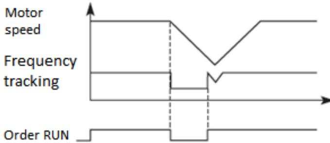
**Warning:** When the drive starts in the start tracking mode, the drive will track the speed in order from high to low frequency.
