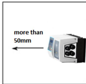
\* Be careful when installing several inverters, install them in parallel and with cooling
