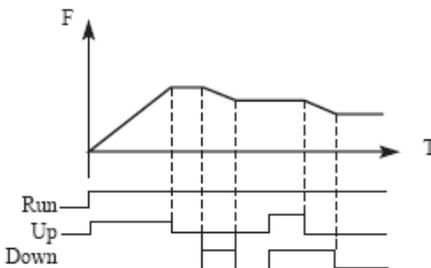
Explanation: if UP is active (UP is closed), the frequency will increase. If DOWN is active (DOWN is closed), the frequency will decrease.
