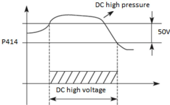
If the value of P414 is too high, the DC voltage may be too high and cause the drive protection to trip. If the value of P414 is too low, the brake resistor may be too hot.
