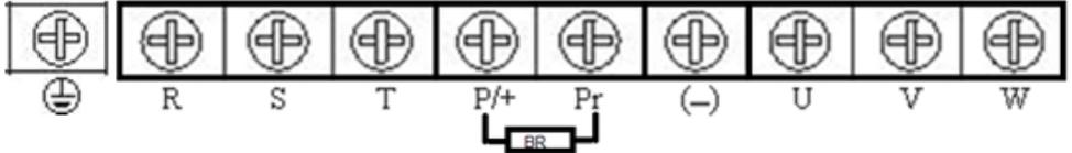
c./ Main terminal block for types powered by 3 x 400 V (690 V), 11 to 15kW with BR.
