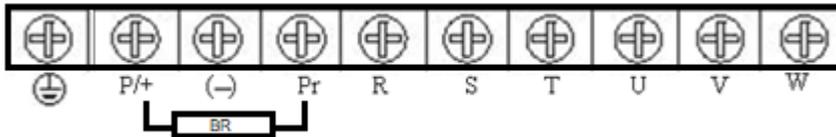
d./ Main terminal block for types powered by 3 x 400 V (690 V), 18.5 to 110kW without BR
