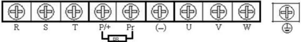
b./ Main terminal block for types powered by 3 x 400 V (690 V), 5.5 to 7.5 kW with BR
