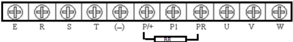
f./ Main terminal block for types powered by 3 x 400 V (690 V), 132 to 315kW
