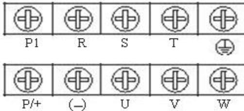
NOTE: "710-1000 kW inverters, top row, front port connection; second row, connection via rear hole".
